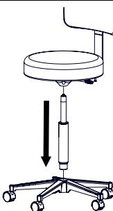
2. Install the larger end of the gas spring into the base of the stool. Place the seat of the stool on top of the gas spring. Sit on the stool to secure the pieces.
