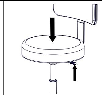
2. To lower the height of the stool, lift up on the lever below the seat while placing weight on the seat.
