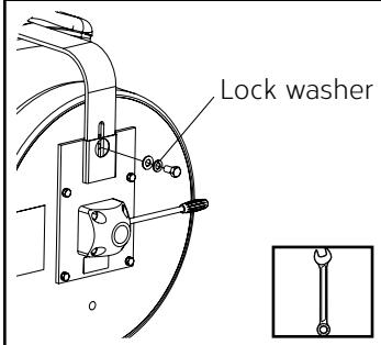
1. Insert the backrest into the bracket on the underside of the seat. Tighten in place with the bolt and two washers.
