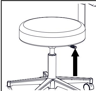
1. To raise the height of the stool, lift up on the lever below the seat with no weight on the seat.
