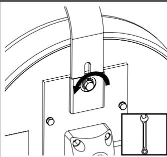
3. To adjust the position of the back, loosen the bolt under the seat, slide the back in or out, and tighten the bolt.
